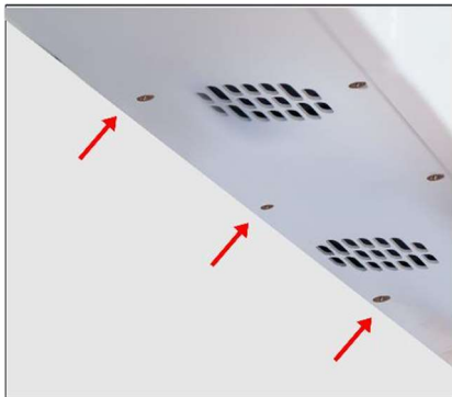
Figure 11 - Sound Deflector Screw Location
