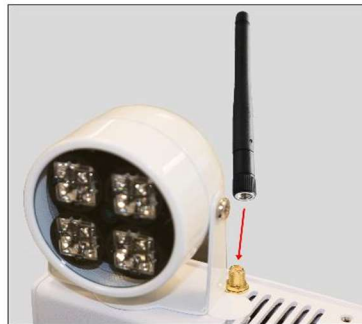
Figure 14 - Installing Wi-Fi Antenna
