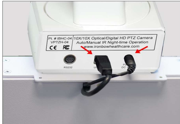
Figure 5 - Connecting the two Camera Cables
