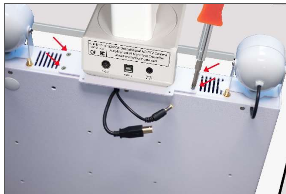
Figure 4 - Attaching Mounting Plate to System Chassis
