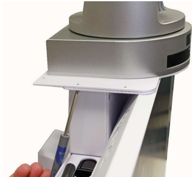
Installing the camera assembly using Philips head screws
