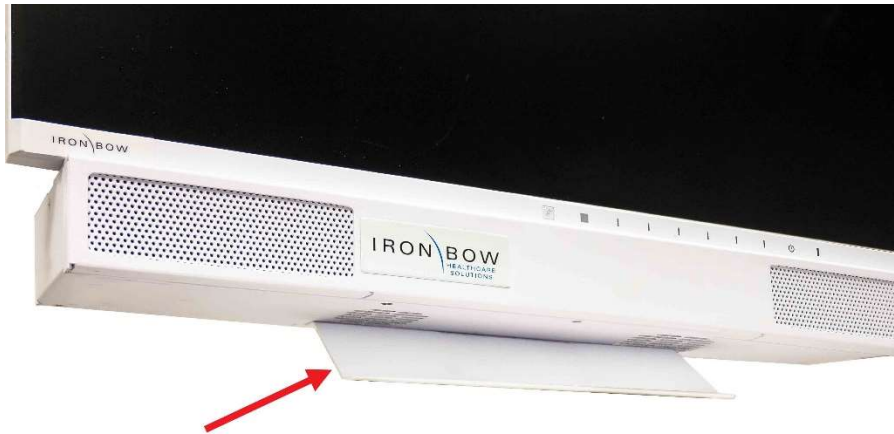
Figure 7 - Sound Deflector Shield
