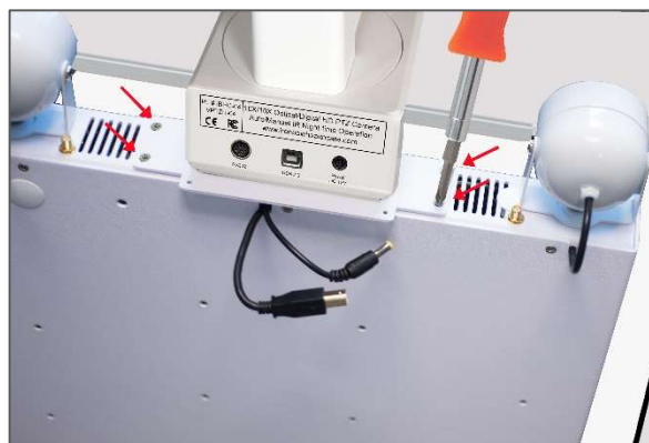
Figure 4 - Attaching Mounting Plate to System Chassis
