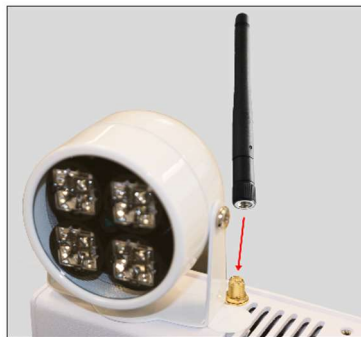
Figure 11 - Installing W-Fi Antennas
