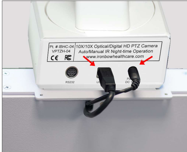
Figure 5 - Connecting the two camera cables
