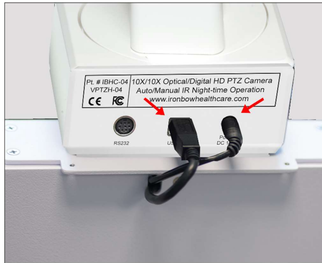
Figure 5 - Connecting the two camera cables
