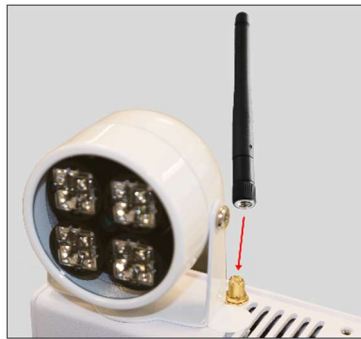
Figure 12 - Installing Wi-Fi Antenna
