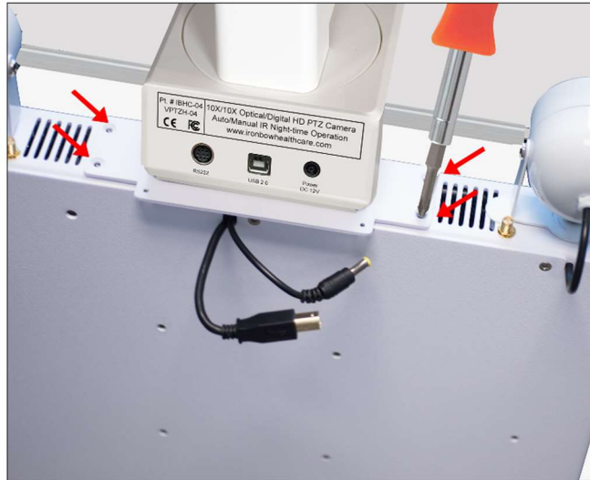
Figure 4 - Attaching Mounting Plate to System Chassis
