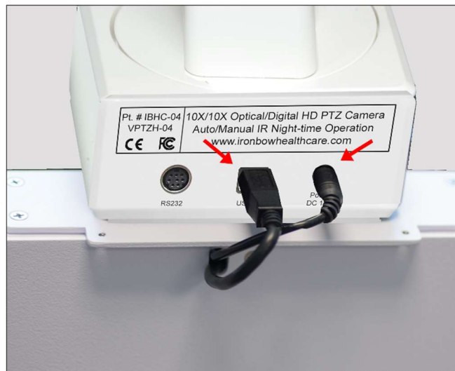
Figure 5 - Connecting the two camera cables
