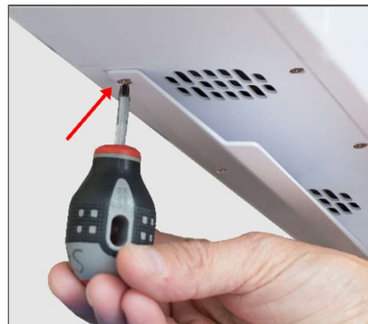
Figure 8 - Installing Sound Deflector
