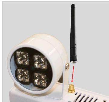
Figure 12 - Installing Wi-Fi Antenna
