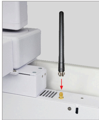
Figure 8 - Installing W-Fi Antennas
