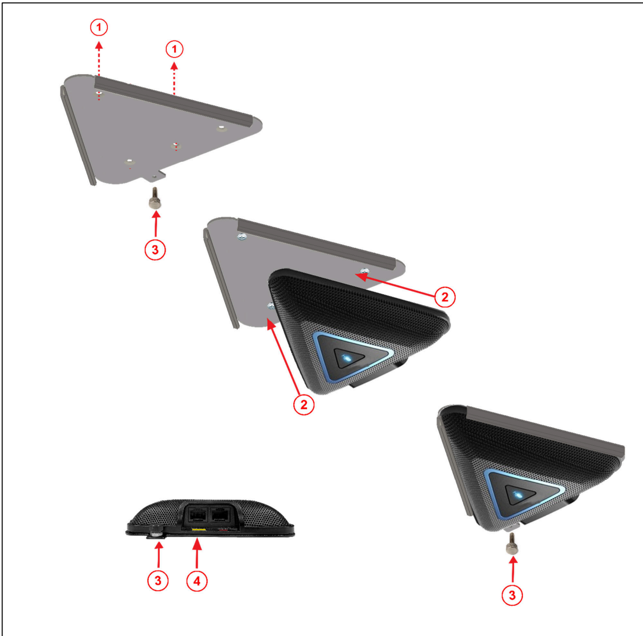
Figure 24 - Installing Ceiling Mic Array
