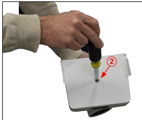
Figure 4. Attaching Camera to Mounting Plate
