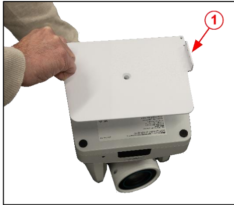
Figure 3. Aligning Camera to Mounting Plate
