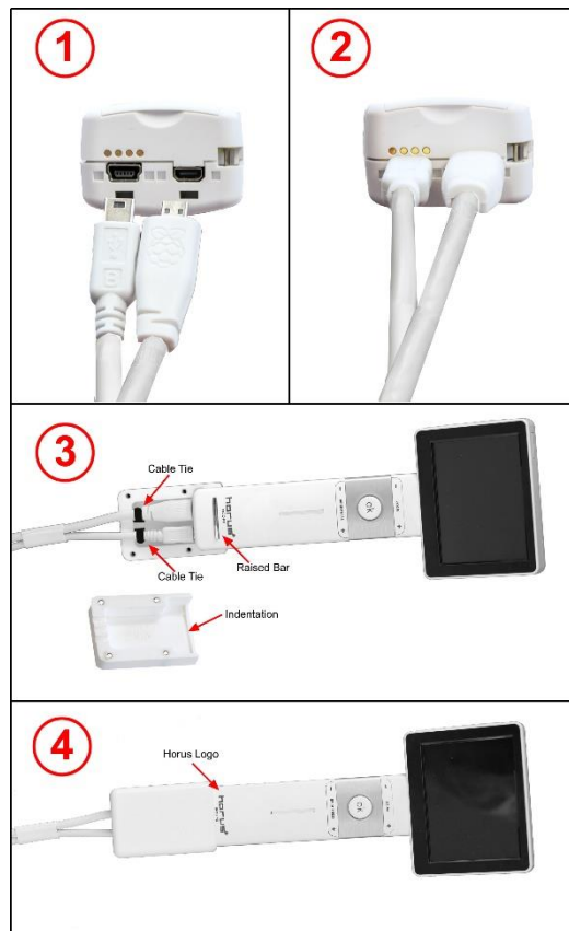
Figure 37. Attaching Cable Clamp
