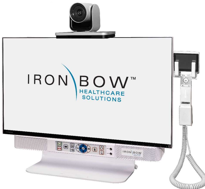
Figure 1. Poly CLINiC pictured with optional desk stand, Horus Scope and Horus Scope cradle
