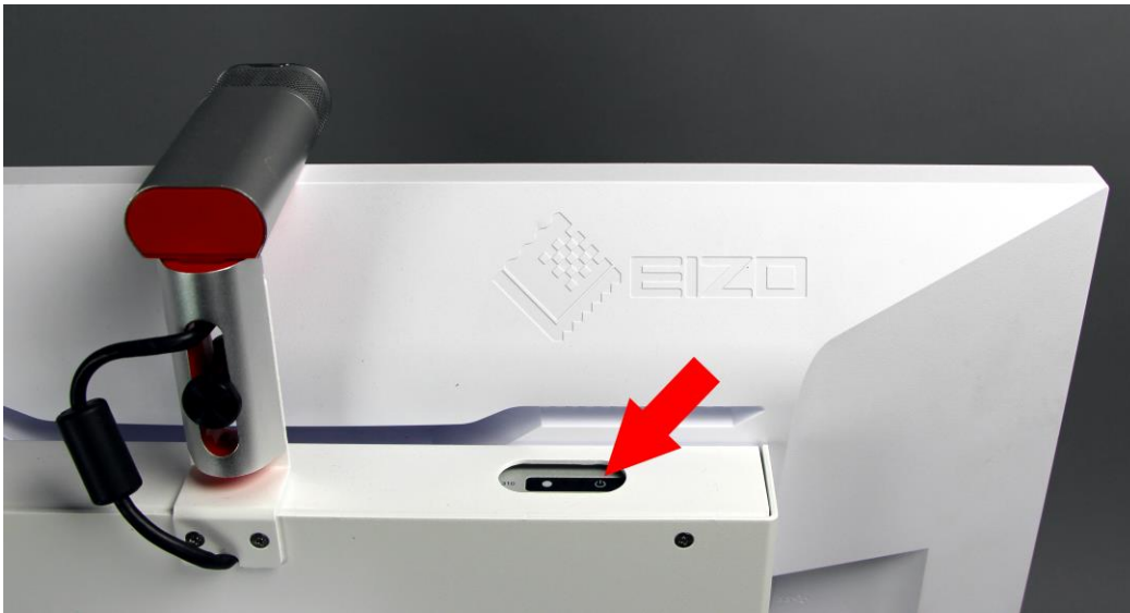
Figure 6. CLINiC 2x rear view with codec power sensor
