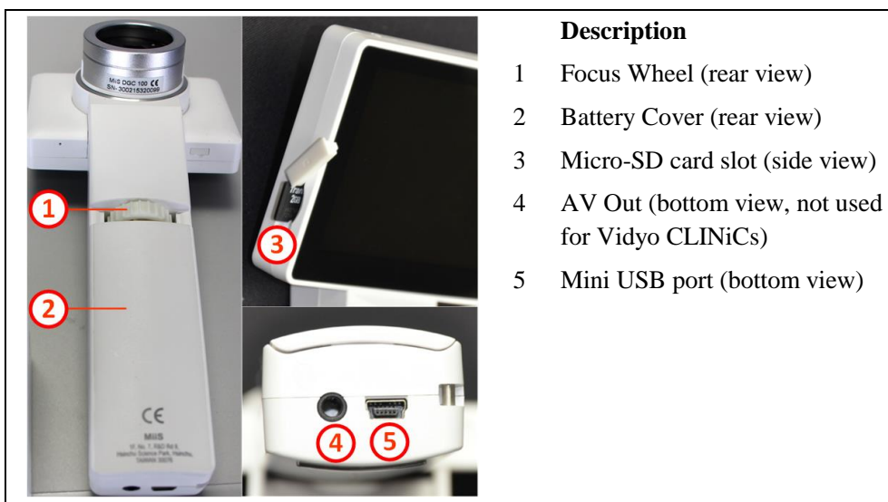
Figure 6. Horus scope components (rear, side and bottom views)
