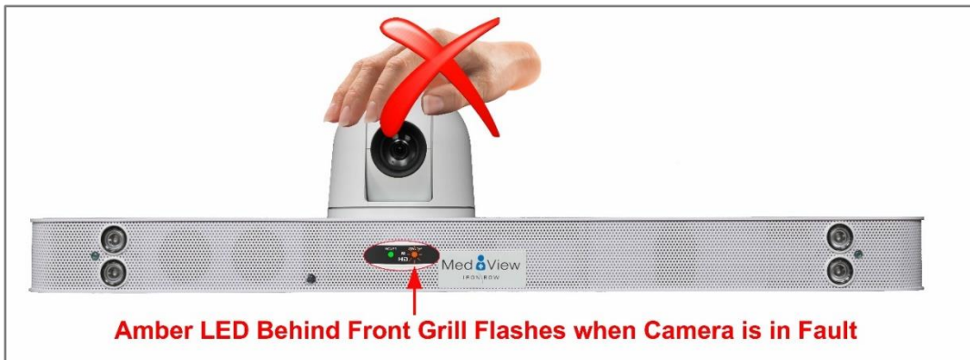
Figure 25 – Camera Fault Condition Indicator
