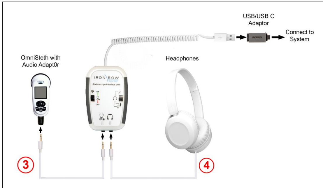
Figure 25. Connecting Stethoscope and Headphones to SIU
